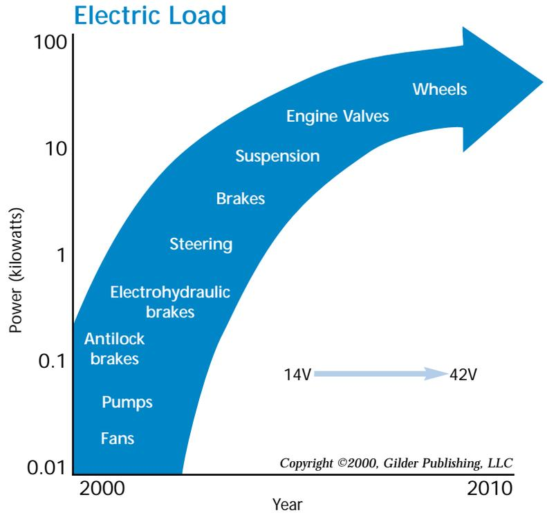
Direct drives take control under the hood, system by system. An integrated starter/alternator displaces existing separate components, and a 42V power bus replaces today's 14V standard. The end point: an all electric powertrain, from wheels to sunroof, headlights to tailpipe.
