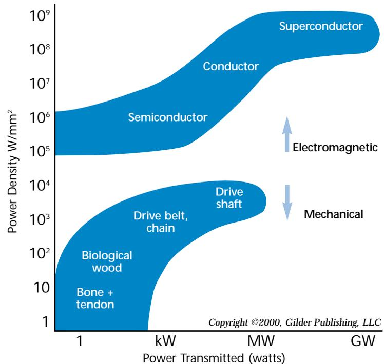
*Power densities in mechanical power trains are ultimately limited by the physical strength of materials and the speed of sound. Power densities in electromagnetic power trains begin two orders of magnitude higher than the highest-power-density mechanical systems, and go up from there. They are ultimately limited by the dielectric strength of the conductor and the speed of light.*
