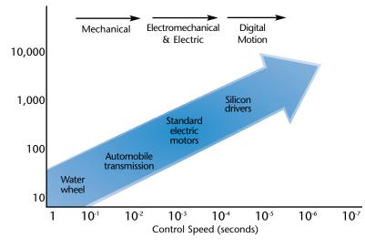
The two overarching trends in motion and control: (1) Higher power density in motors and converters; (2) Faster controllers, that provide more precise control.
