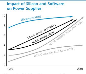
Driven by the triad of better silicon, sensors, and software, power supplies have achieved record densities (DC-DC now hitting 100 W per W/in<sup>3</sup>, AC-DC beyond 10 W/in<sup>3</sup>), greater efficiency (up more than 10 percentage points in the decade), and greater reliability (AC-DC now over one million hours mean-time-between-failures (MTBF), and DC-DC over 40 million hours MTBF). All this while costs have dropped four-fold in dollars per watt. The trend continues.
