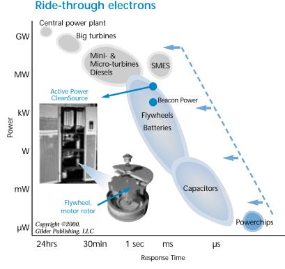
Powercosm technologies span a wide range of power levels and response times. Batteries, and now flywheels, provide ride-through power in the middle of the curve, where substantial amounts of power are required very fast, to keep racks of silicon lit during the grid's frequent dips.
