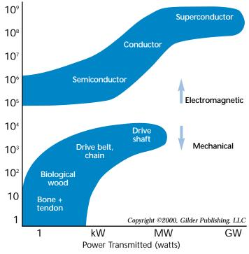
Power densities in mechanical power trains are ultimately limited by the physical strength of materials and the speed of sound. Power densities in electromagnetic power trains begin two orders of magnitude higher than the highest-power-density mechanical systems, and go up from there. They are ultimately limited by the dielectric strength of the conductor and the speed of light.
