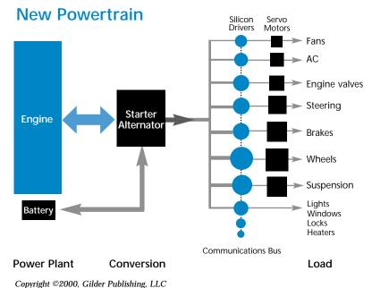
An integrated electrical power transmission system, terminating in silicon drivers and servo motors, interconnects by way of a digital communications bus. The intelligence is lodged in
